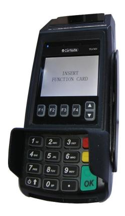
Cartadis TLC6N reloads contactless cards or creates wash codes used on the TL12 terminal to control a gantry. The TLC6N equipment is also compatible with the DJ3 token dispenser, the TL14 terminal and the TCM2-CHSP reader for high pressure and vacuum terminals.
